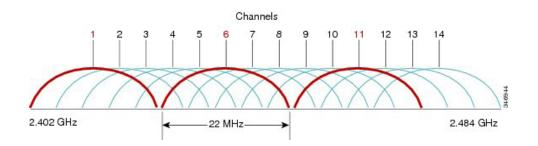
Non-overlapping channels must be used and allow at least 20 percent overlap with adjacent channels when deploying Cisco DX650 in the 802.11b/g/n environment, which allows for seamless roaming.
