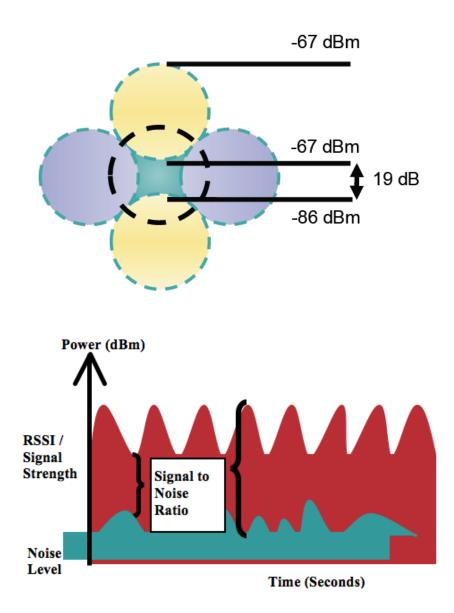
When designing the placement of access points, be sure that all key areas have sufficient coverage (signal).
