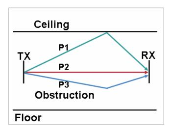
Use of Orthogonal Frequency Division Multiplexing (OFDM), which is used by 802.11a and 802.11g, can help to reduce issues seen in high multipath environments.
